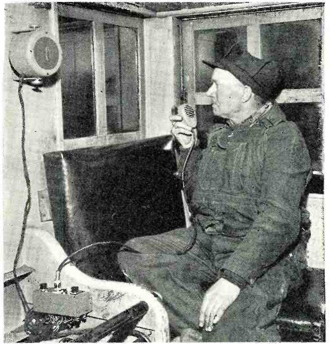
Railroader tests the installation from the caboose. The speaker and remote-control panel may be seen at the left.
