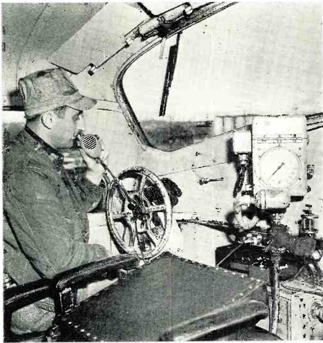
Fireman of the "Flying Ute" talks to the conductor via FM radio during test of locomotive-to-caboose communications.
